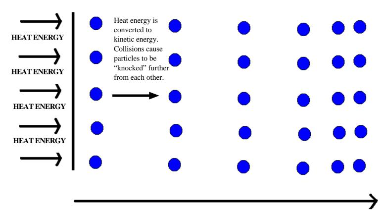
Particles nearer the heat source speed up causing collisions and increasing distance between particles. Further from the source, the energy is reduced, decreasing the distance between the particles. As the heat energy applied increases, the further from the source this energy is distributed.
