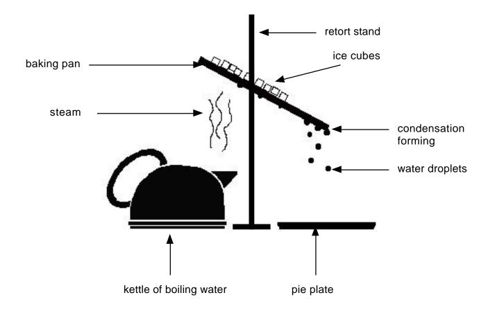
Note: Pouring the water that collects in the pie plate back into the kettle completes the cycle. Ask the students if they know what part of the cycle this represents (runoff).
