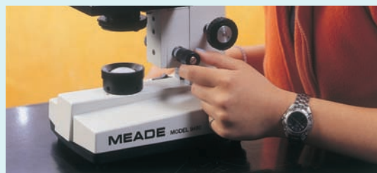
Figure 1.8 The fine adjustment knob brings the object into sharper focus.
